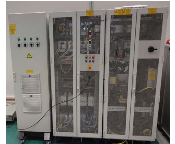
Three-phase asynchronous motor emulator for frequency converter load testing
