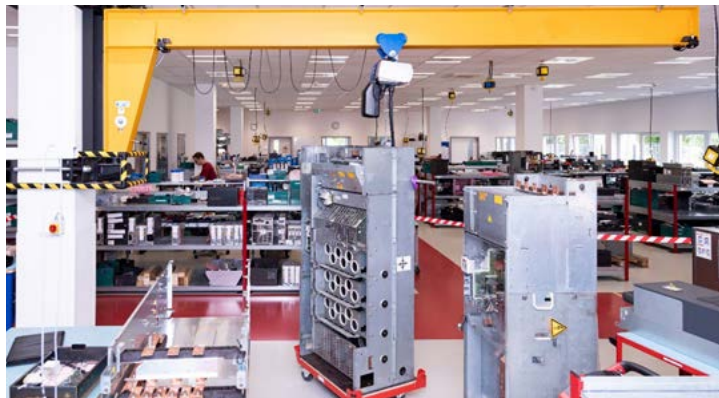
Fig. 3: Large inverter and cabinet-mounted inverter in the EICHLER repair workshop
